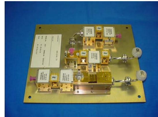
94 GHz upconverter and downconverter prototype for military FMCW application
