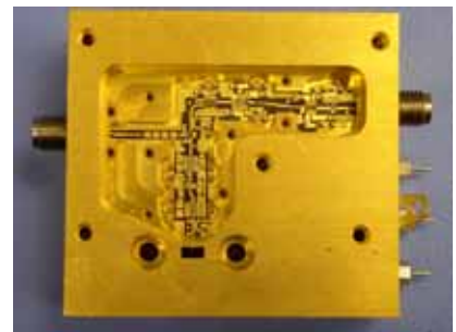
60 GHz Integrated Receiver
