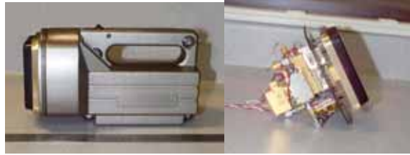
HXI's first radar product: a 60 GHz hand-held, concealed weapons detector developed for law-enforcement personnel (top left: complete unit; top right: 60 GHz radar front end).
