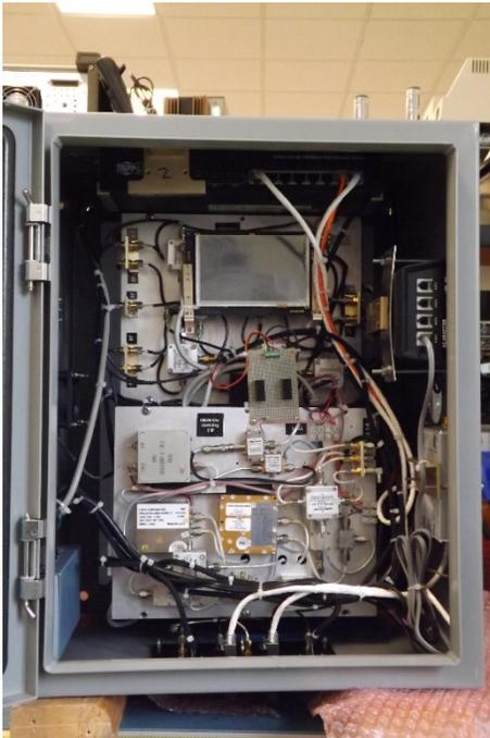
94 GHz FOD Radar Electronics Enclosure
