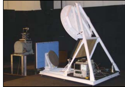
Compact Antenna Range (30" x 20" Quiet Zone, operates to 100 GHz)
